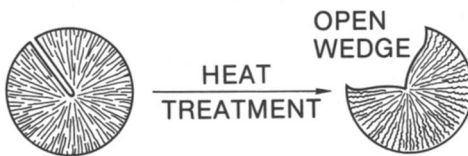
Figure 2. Mesophase carbon fiber with radial structure and open-wedge shape. Polarized light.
