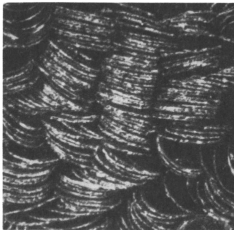
Figure 5. Model of distorted columns formed by BSU's (23).
