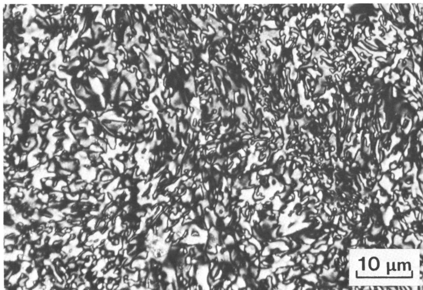
Figure 4. Optical micrograph of a coke surface showing an optical texture of medium- and coarse-grained mosaics, 1.5 - 10 \mu\text{m} diameter, OTI = 5.
